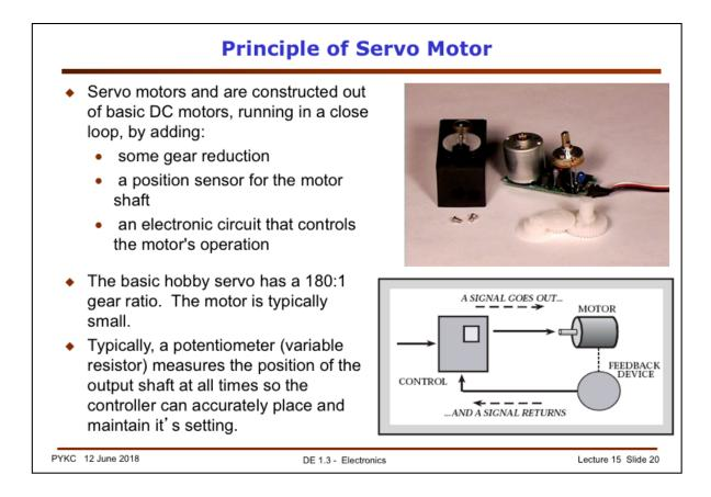
Finally, we will consider a type of motor which is really a DC motor put into a control feedback loop. This is the servo motor.
