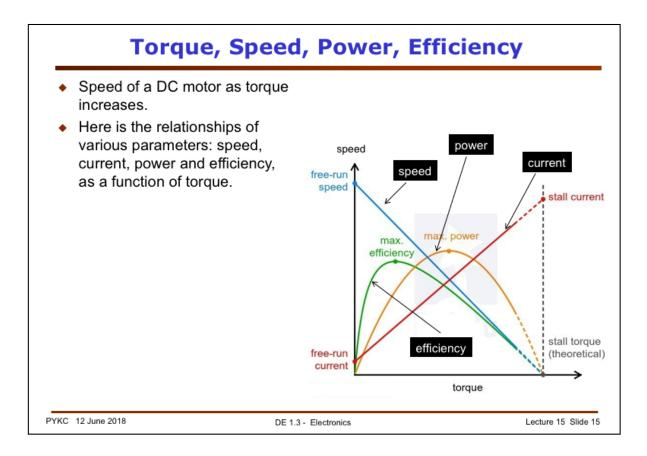
In consider which motor to use, you need to examine the way speed changes with torque. In DC motors, the torque drops with increasing speed. Hence you get the power and efficiency curves as shown. There is a maximum power (transferred) and maximum efficiency point at some torque level. The datasheet of the motor will always specify this.
