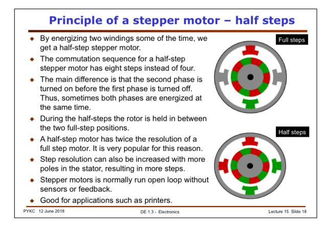
Stepper motors can be controlled in full steps. However, by pulsing the neighbour earlier (i.e. between phases), we can move the rotor to the half way point as shown in the animation here. This is called the half-stepper.
