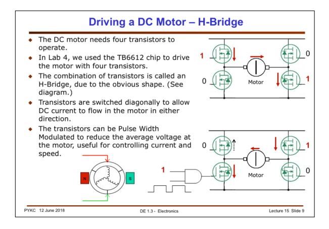
Since motor coils are essentially inductors, they have low DC impedances (resistance of the wiring). Hence when driving motors, we need to use special driver chips.
