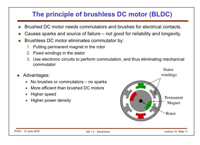
Brushed DC motors are cheap to make and simple to use – apply a DC voltage, such as connecting it to a battery, or drive it with PWM, you are ready to go.
