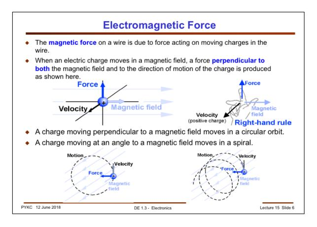
If you have a current carrying conductor moving through a magnetic field, or moving a magnet near to a current carrying conductor, a force is produced. The direction of the force is perpendicular to BOTH the magnetic field and the electric current, as governed by the Right-Hand Rule shown above. (You probably have done this in high school physics.)
