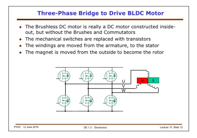
Here we see the transition from DC to Brushless DC motors. Especially the replacement of the brushes and commutators with the six transistor (three-phase) bridge.
