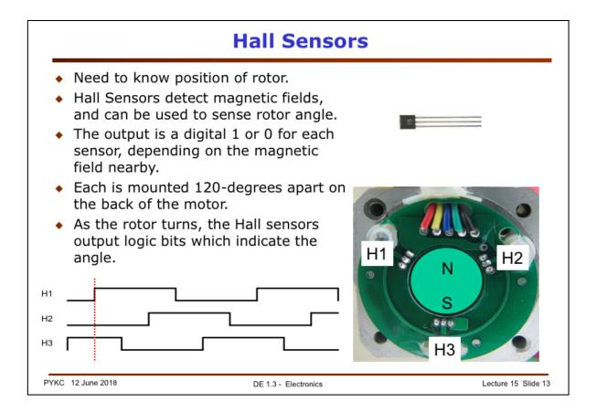
Since we can performing commutation electronically, we need to synchronise the driving signal to the rotor position. In other words, we need to SENSE the position of the permanent magnets on the rotor. This is achieved by the Hall Effect Sensors.
