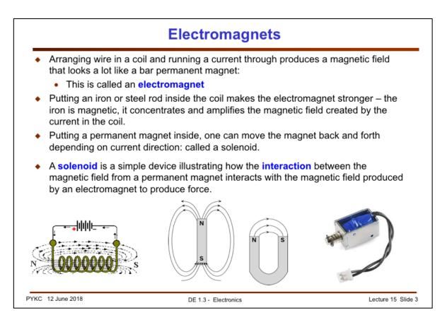
If we wind a coil of wire around a tube, and then pass current through the coil, we have an electromagnet that behaves like a permanent magnetic with a north and a south pole. Removing the current, this is just a coil of wire – all the magnetic filed will disappear. This is called an electromagnet.
