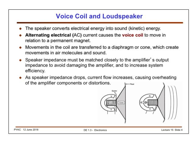
An other good example of application of electromagnet is the loudspeaker.
