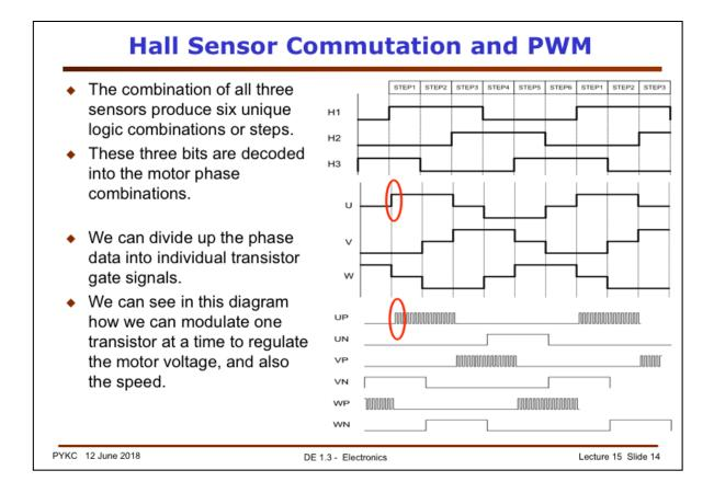
You can take the three Hall signals as digit bits, and assign them a number, based on their binary states. You could say that step 1 is binary 101, step 2 is 001, etc. Filling in a table of 6 combinations, plus the two other invalid states of 000 and 111 gives all the combinations. Then, let the U-phase upper transistor be ON when the Halls are equal to 001 (decimal 1) or 101 (decimal 5).
