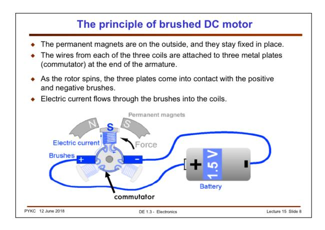
This slide shows how a DC voltage source is applied to different coils to produce an electromagnet in the rotor. This electromagnet interface with the permanent magnets in the stator – thus producing rotational motion.
